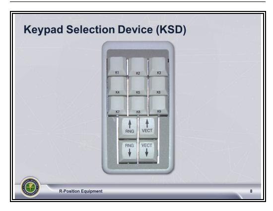
The Keypad Selection Device (KSD) may be located anywhere on the radar console or the corresponding RA console, and allows quick access to functions on the R-Position console without using the trackball or keyboard.
